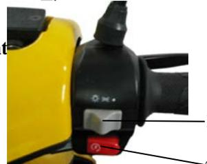
When it on (☺) position taillight, position Light and instrument turn on.
